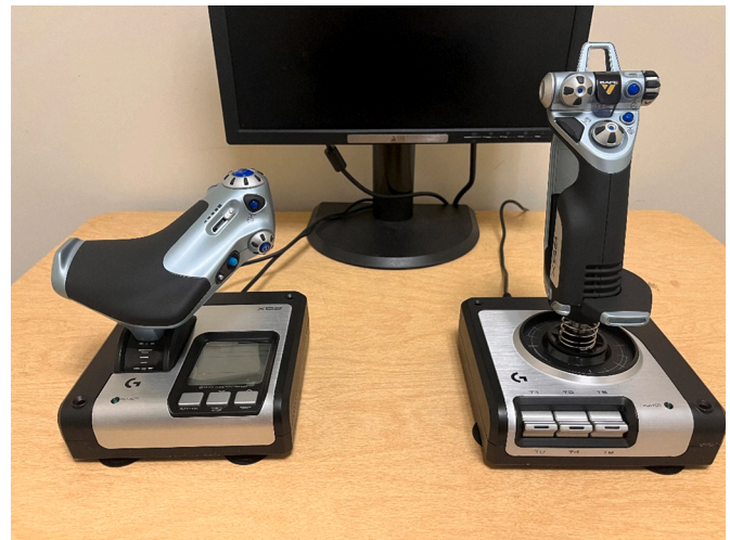
Fig. 6. The hands-on-throttle-and-stick controllers used for the performance based measures.
